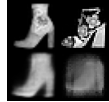
Figure 3: Reconstruction of a shoe from Fashion-MNIST using (left) a standard VAE, and (right) the VAE architecture of [2]. Both networks have the same depth and layer widths where possible, as well as the same activation function, to ensure a fair comparison.
